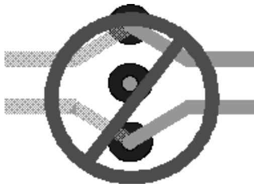
Figure 8-4. No Vias Between High-Speed Traces
