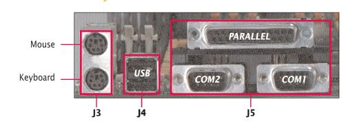
Note: On UP2000-A3 boards and above, COM1 port is reserved for a serial remote console device.
