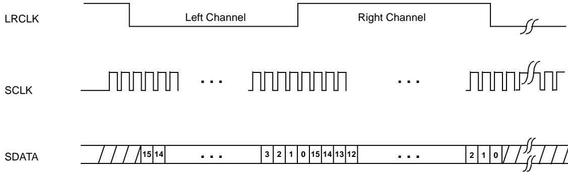
Figure 24 I<sup>2</sup>S Digital Input Format
