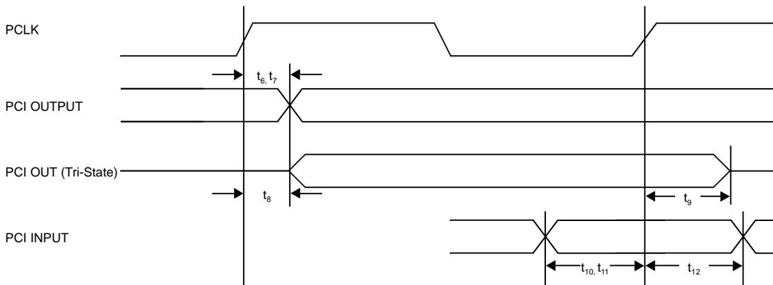
Figure 17 PCI Signal Timing<sup>1</sup>
