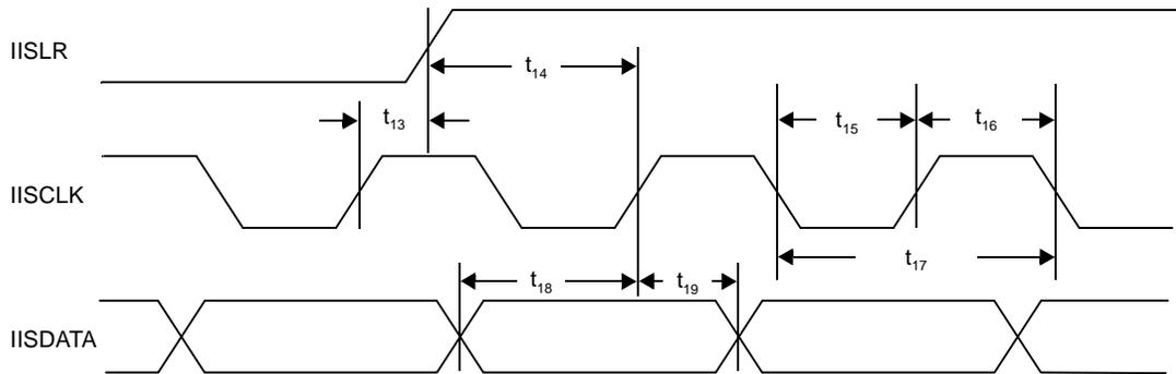
Figure 18 Serial Input Timing for I<sup>2</sup>S Interface
