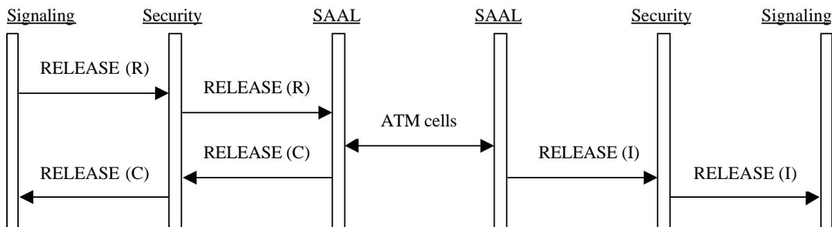
**Figure A-4: Connection Termination With No Data Transfer.**
