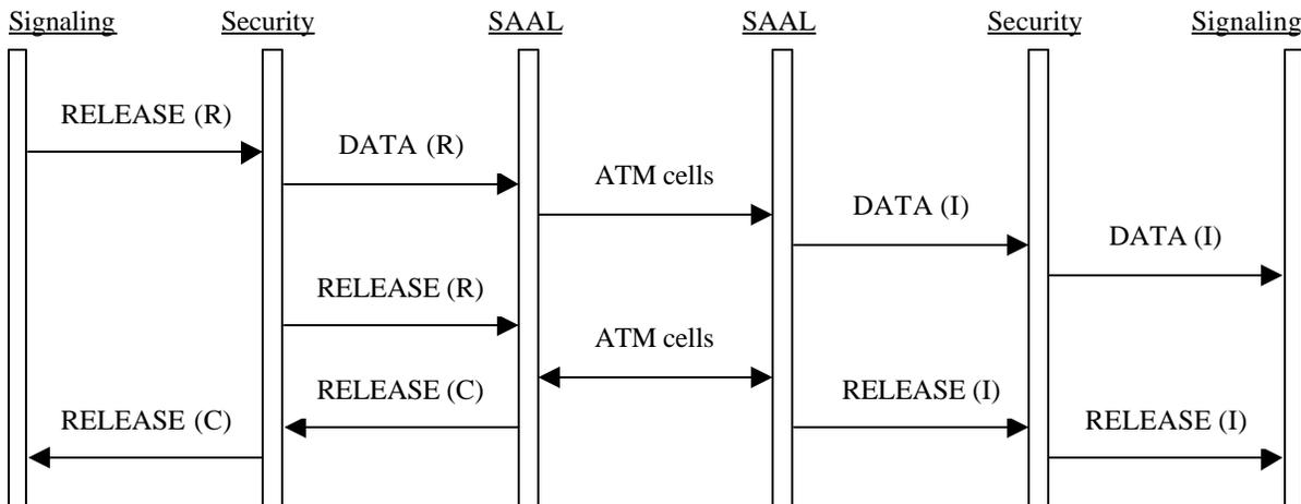
**Figure A-5: Connection Termination With Data Transfer.**
