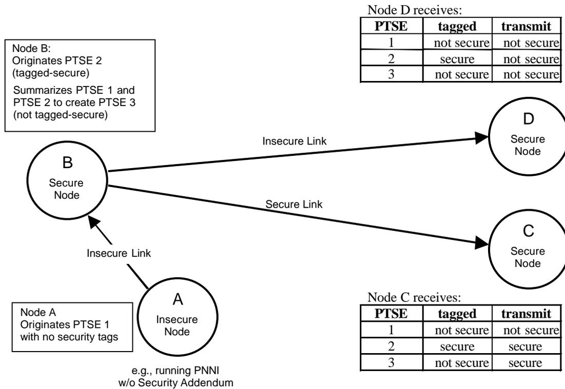
**Figure 8: Tagged-Secure and Transmit-Security Example.**
