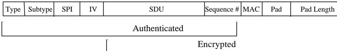
**Figure 4: Frame Format for Control Plane Security.**
