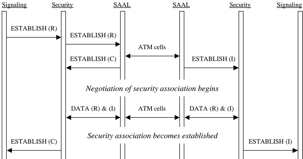
**Figure A-1: Connection Establishment With No Data Transfer.**
