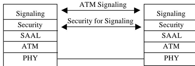
**Figure 2: Reference Model (Signaling).**
