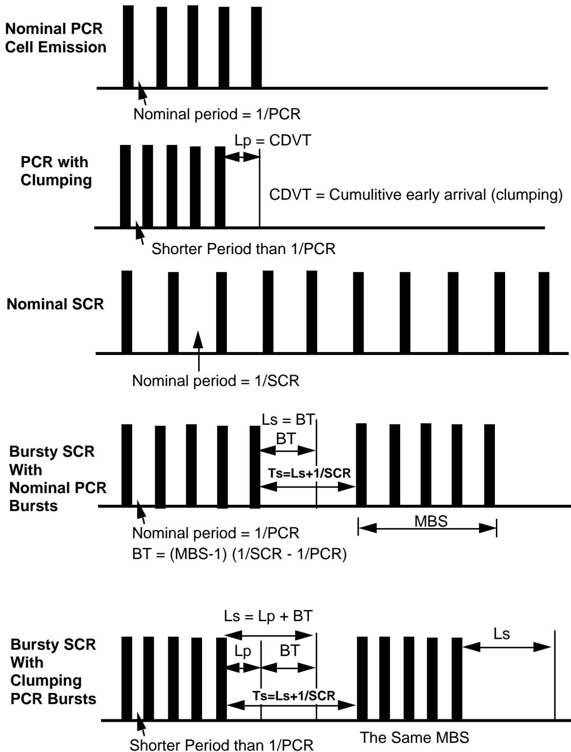
Figure 9.2 Illustration of Traffic Shaping Requirement in the FUNI IWF
