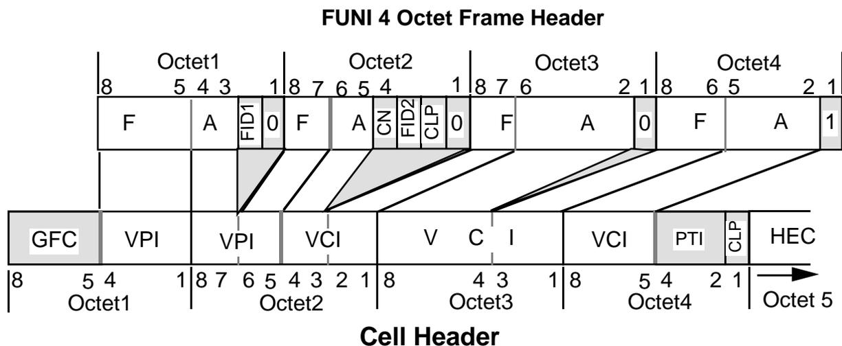
**Figure 3.7 Mapping Between the Frame Address (FA) and VPI/VCI Fields for Four Octet Header Frames**
