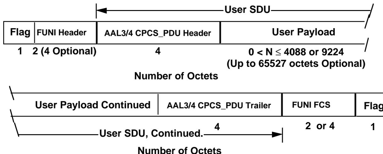
**Figure 3.1 Illustration of FUNI SDU/AAL3/4\_CPCS\_PDU Encapsulation in a FUNI PDU**
