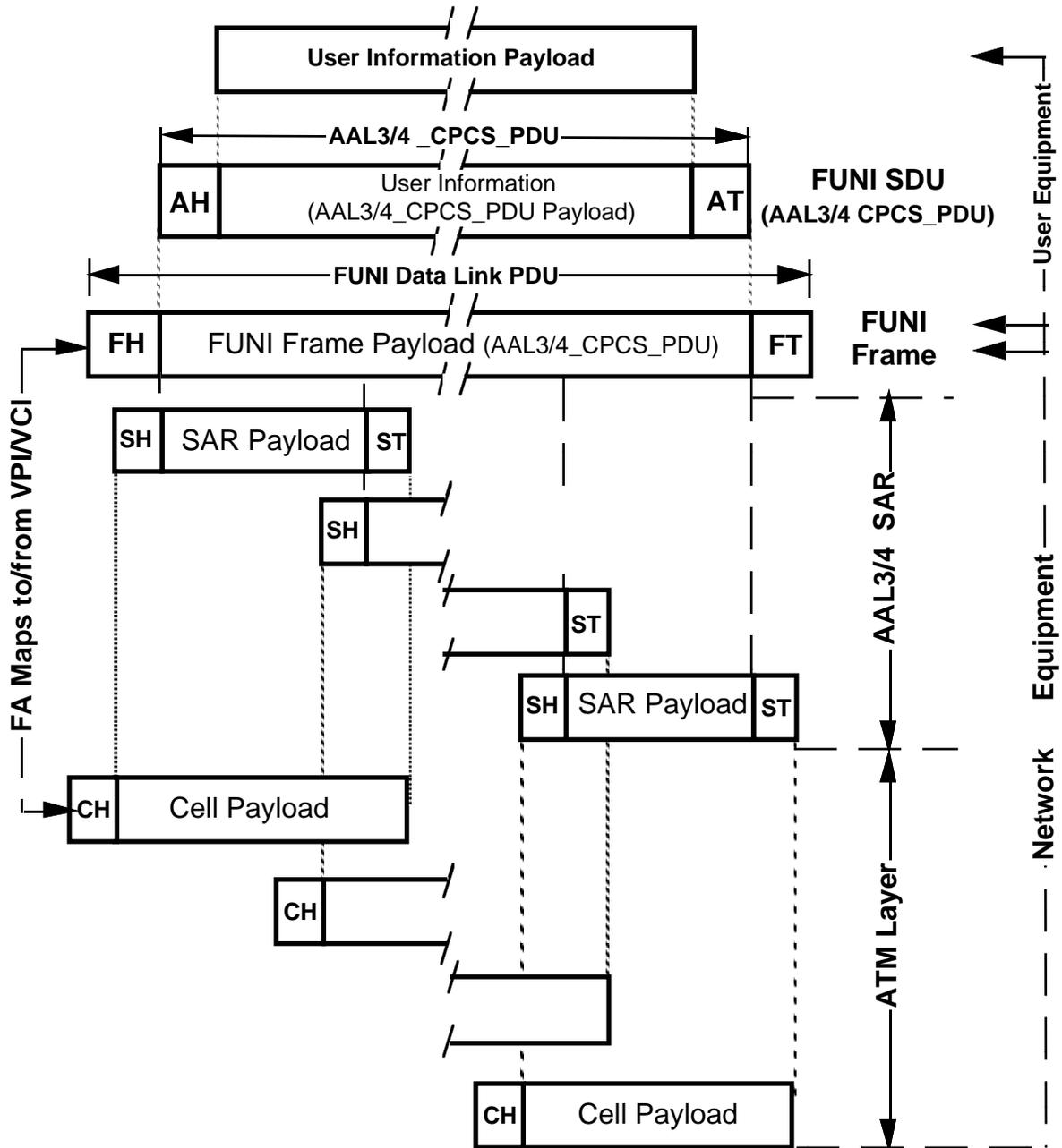
FH = FUNI Frame Header      FT = FUNI/HDLC Frame Trailer      Note: HDLC Flags are not shown
