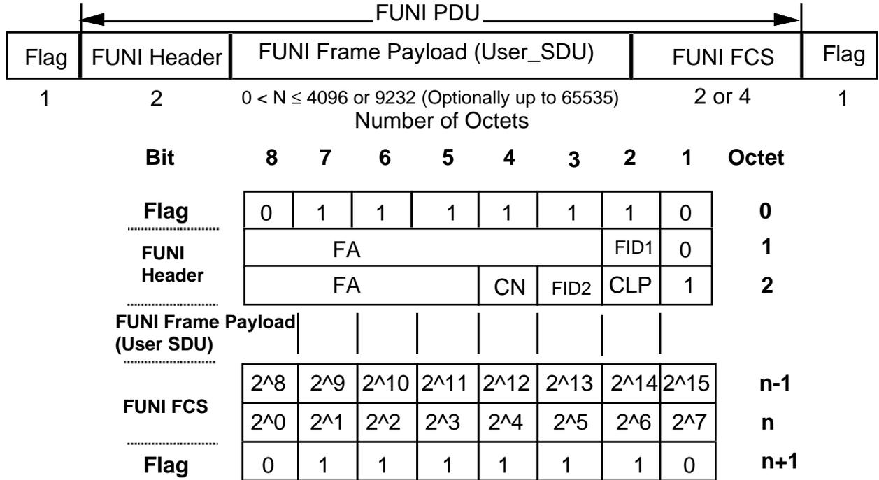
**Figure 3.4 FUNI Frame Format for the 2 octet Header Frames (shown with a 16 bit FCS)**
