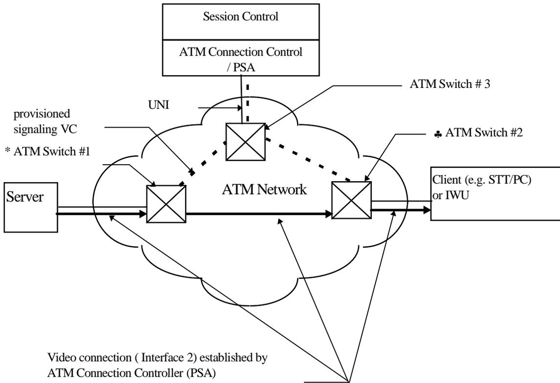
\* Signaling endpoint is ATM Switch #1
