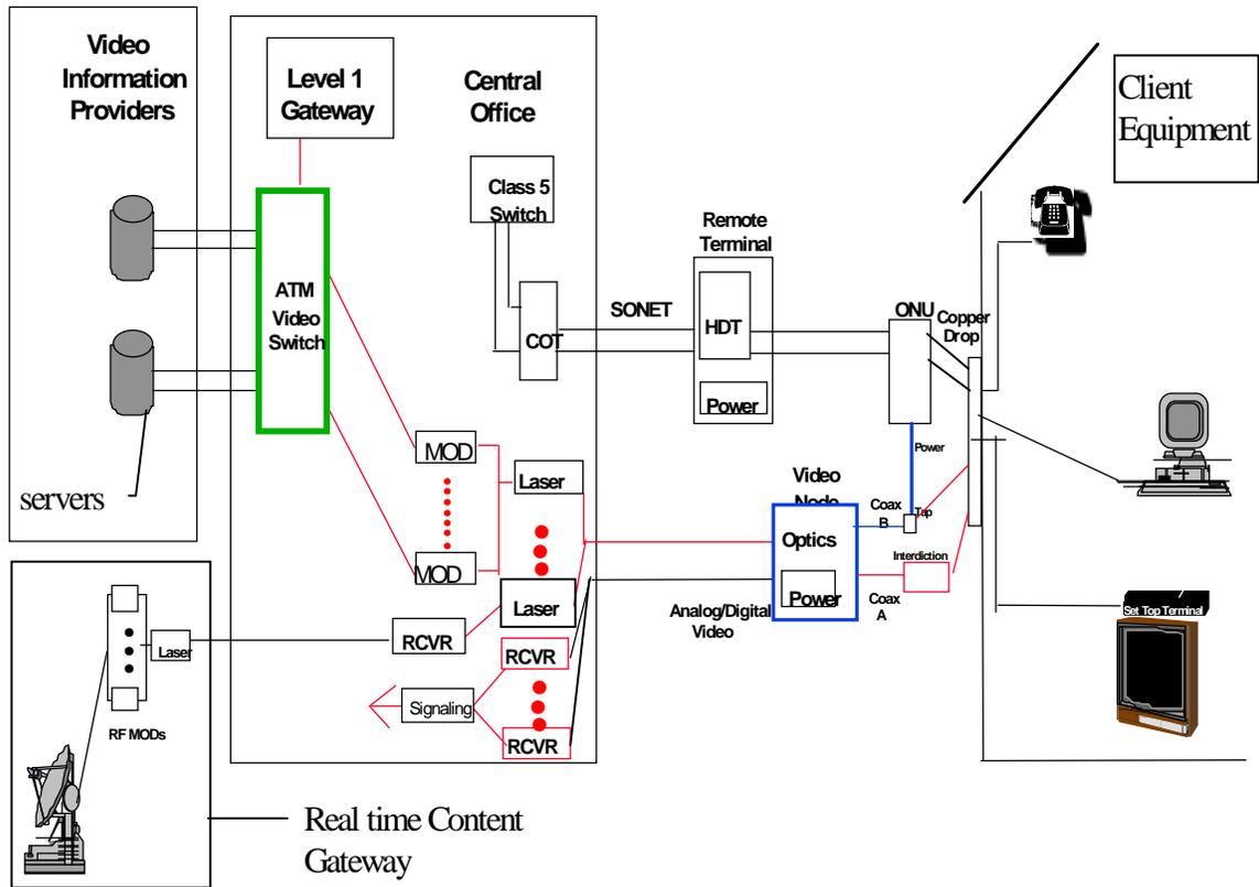
Figure B-1 Hybrid Fiber Coax Network VoD Example
