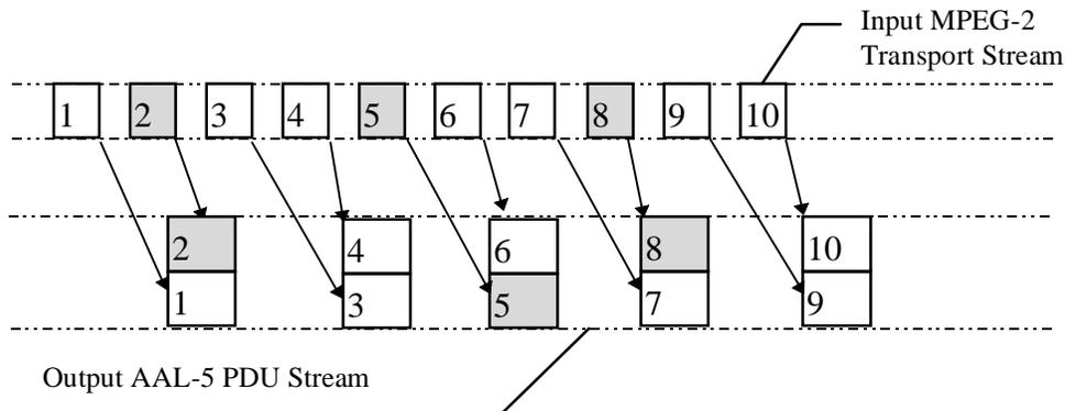
Figure A-6 Example Non-Alignment of MPEG-2PCRs with AAL5 PDU Boundary
