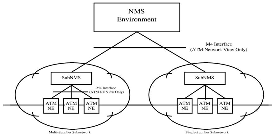
**Figure 3-2-1: Example of Network-View Management Physical Configuration**
