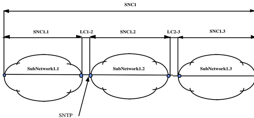
Figure 6.3.2.2-a: Network Transport Architecture
