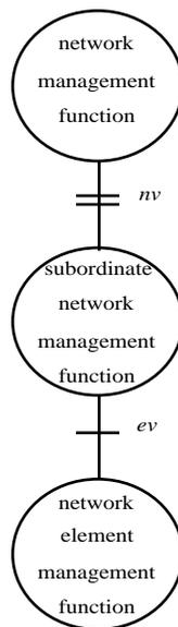
**Figure 3-1: M4 Network-View Logical Architecture**
