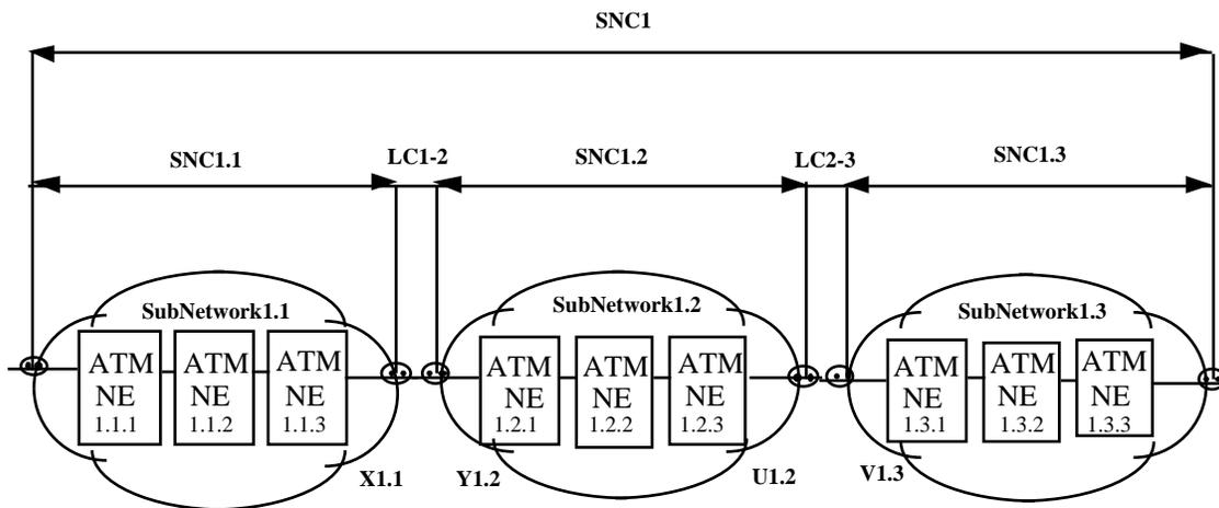
Figure 6.2.3.2-a: Network Transport Architecture
