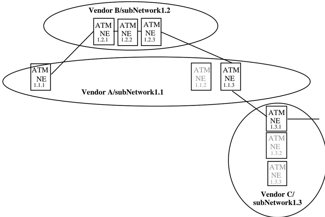
Figure 6.3.3.2-a Network Transport Architecture
