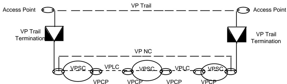
Figure 2 ATM VP Layer Network
