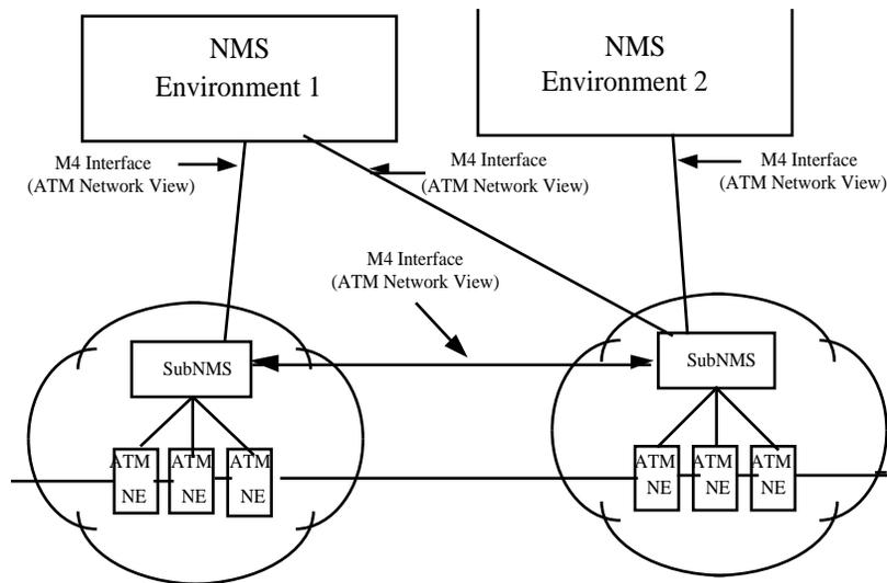
**Figure 3-4-2: Example of Multi-Manager Management Physical Configuration**
