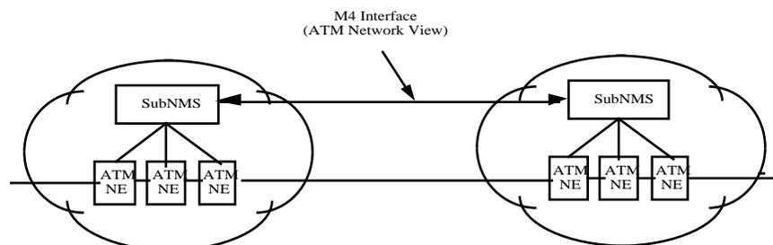
**Figure 3-4-1: Example of Non-hierarchical Management Physical Configuration**
