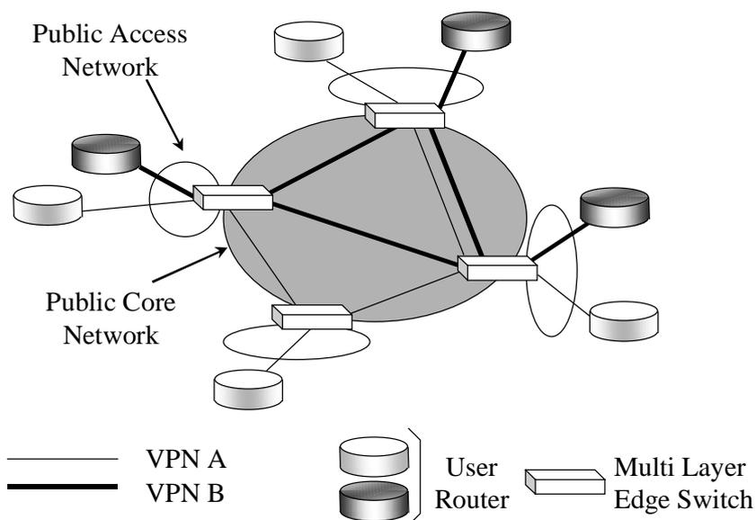
Figure 1: An Example of a Multi Layer VPN
