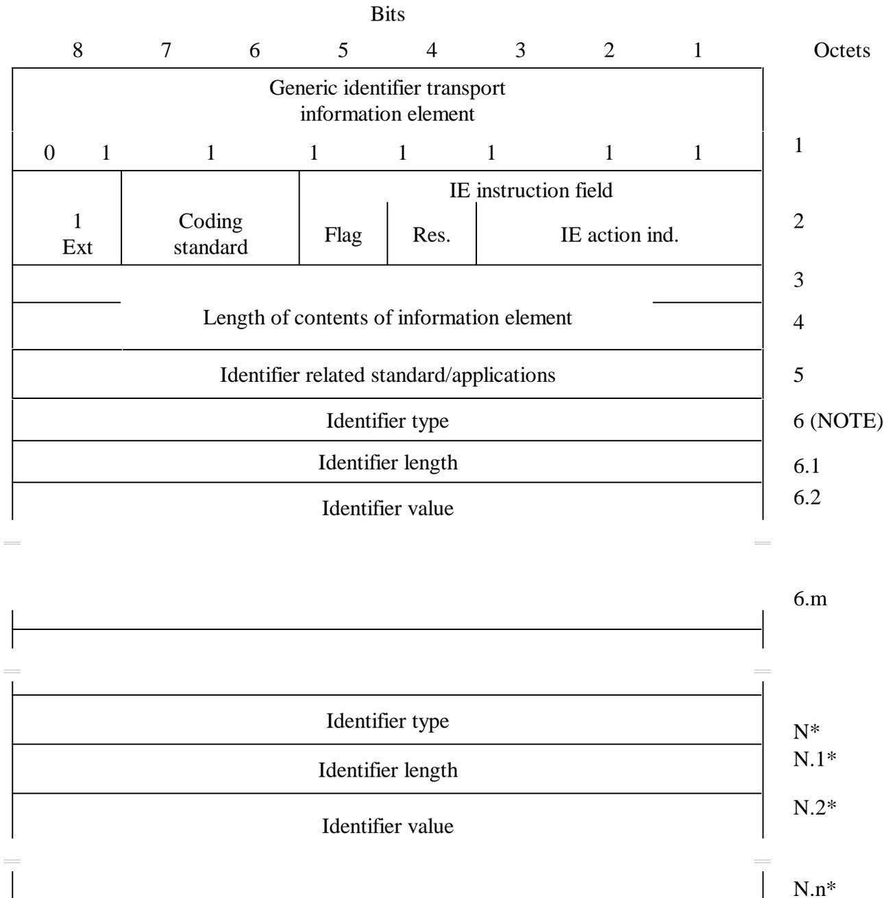
Figure 6: Coding of the GIT Information Element
