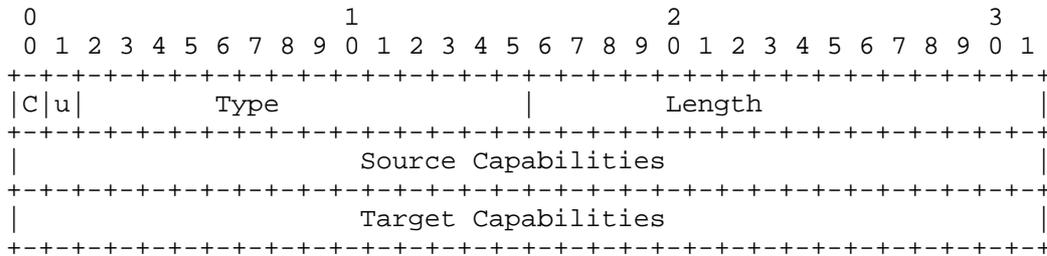
Figure 4: NHRP VPN Capability Extension Format
