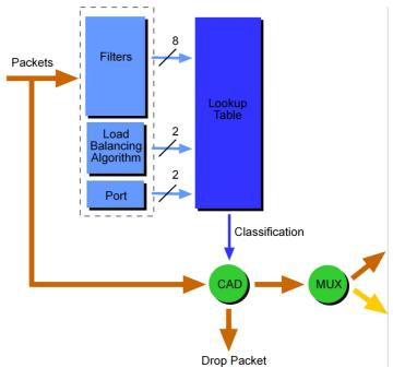
Packets are received from the line and stamped with an ERF (Endace Record Format) header, then past along to the filter and load balancing block.
