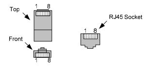
Figure 6-1. RJ45 Plug and Socket Connector Pin-outs.
