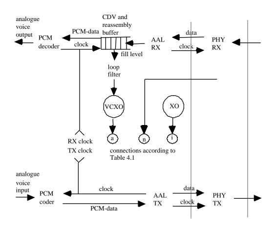
Figure 4-3 Timing relationships in the B-TE
