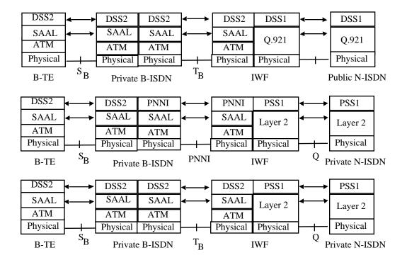
Figure 3-4 Signalling (C-plane)
