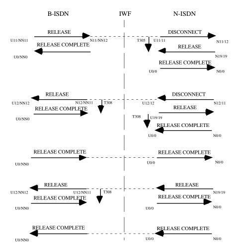
Figure 3-5 Mapping of call clearing messages
