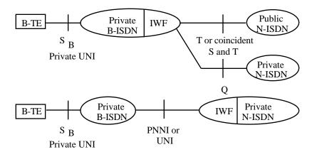
Figure 3-2 Additional interworking configurations for integrated IWF
