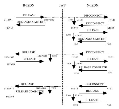
Figure 3-6 Mapping of call clearing messages with collision
