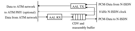
Figure 4-2 Basic structure of the IWF
