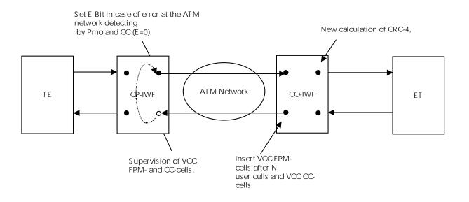
Figure 17: supervision of ATM network by VCC PMo and CC on ATM<sub>down</sub> of CP-IWF
