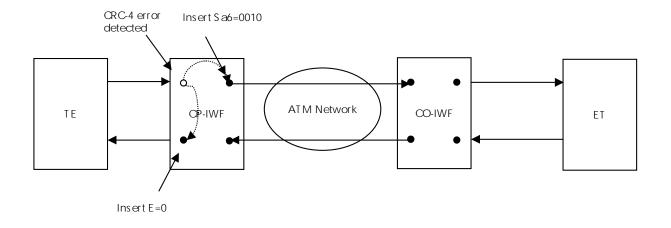
Figure 19: CRC-4 error detected on the  $T_{\rm up}\, signal$  of CP-IWF
