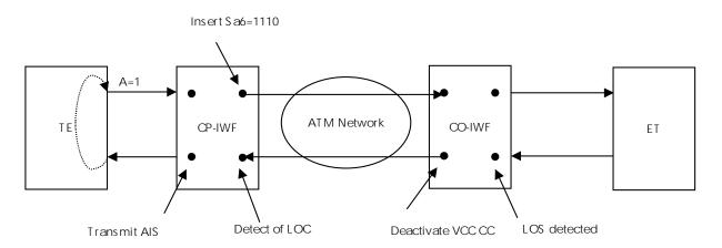
Figure 24: ATM connectivity fault of  $\mbox{ATM}_{\mbox{down}}$  caused by LOS at the CO-IWF
