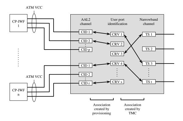
Figure B-2: Relationship between AAL2 channels, CRVs and timeslots in GR-303 CO-IWF
