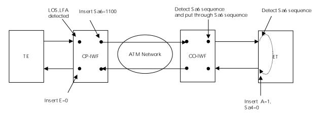
Figure 22: LOS,LFA detected at the  $T_{\rm up}$  interface of CP-IWF
