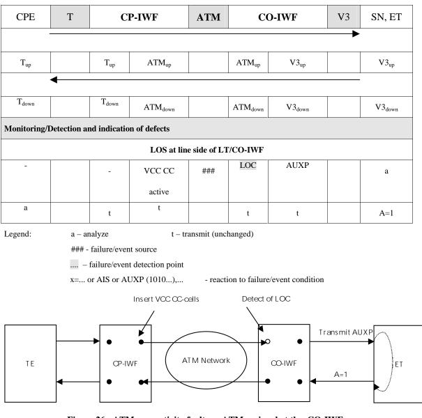
Figure 26: ATM connectivity fault on  $\text{ATM}_{up}$  signal at the CO-IWF
