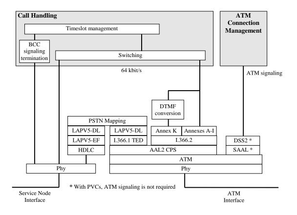
Figure C-1: Protocol Reference Model for CO-IWF with V5.2, using CCS
