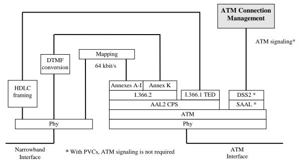
Figure 5: Protocol Reference Model for CP-IWF with ISDN BRI or ISDN PRI user side interfaces with DSS1 relay over AAL2 between IWFs
