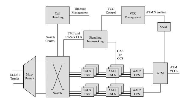
Figure A-1: Example of functions within a CO-IWF
