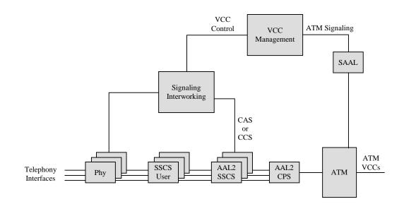
Figure A-2: Example of functions within a CP-IWF
