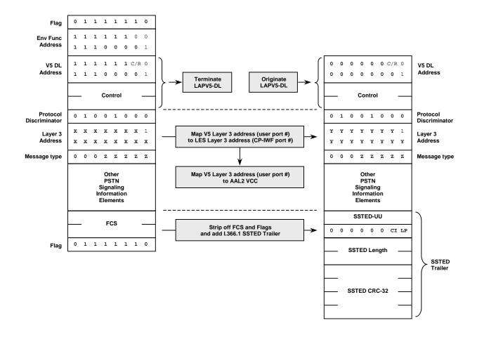
Figure C-2: PSTN mapping function in the direction from network to user
