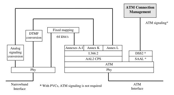
Figure 3: Protocol Reference Model for CP-IWF with analog telephony user side interfaces with CAS transported over AAL2 between IWFs
