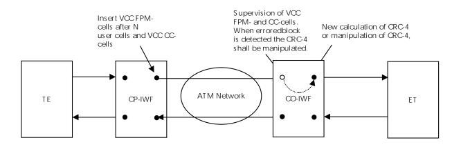
Figure 18: supervision of ATM network by VCC PMo and CC on ATM<sub>up</sub> of CO-IWF
