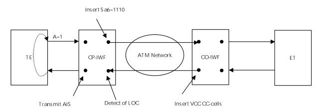
Figure 23: ATM connectivity fault of  $\mbox{ATM}_{\mbox{down}}$  detected at the CP-IWF
