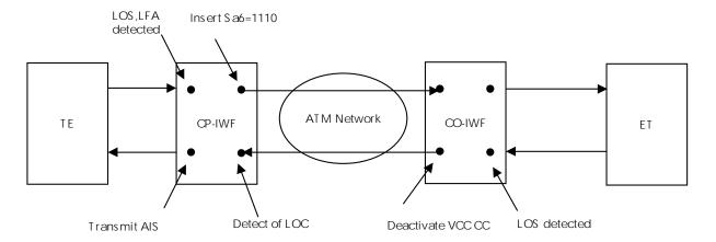
Figure 25: LOS/LFA at T reference point of NT1/CP-IWF AND LOS at V3 reference point of LT/CO-IWF
