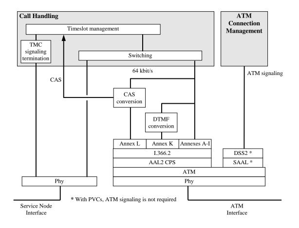
Figure B-1: Protocol Reference Model for CO-IWF with GR-303, using CAS
