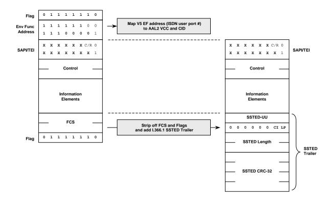
Figure C-4: DSS1 message relay function in the direction from network to user
