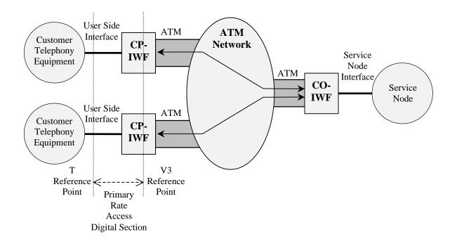
Figure 14: Remote Access Service Deployment Model for ISDN PRI
