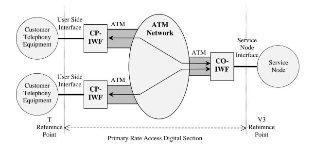
Figure 13: Direct Access Service Deployment Model for ISDN PRI
