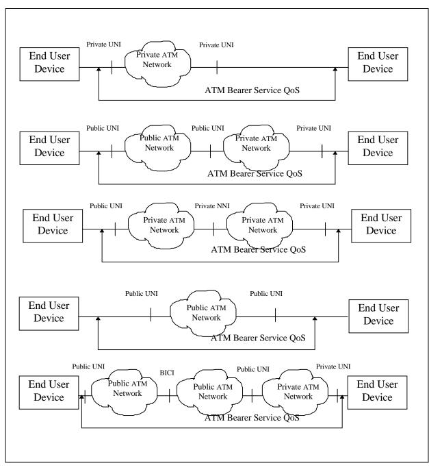
Figure 3-1: ATM QoS Reference Configurations
