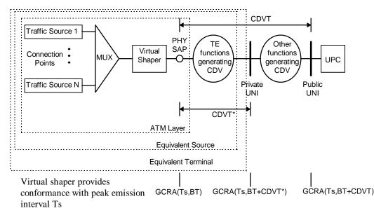
Figure 4-3: SCR and BT Reference Model
