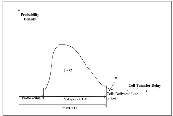
**Figure 3-2: Cell transfer delay probability density model (for real-time service categories)** The components of the fixed delay include propagation through the physical media, delays induced by transmission system, and fixed components of switch processing delay. CDV is induced by buffering and cell scheduling.
