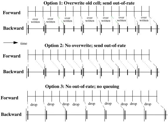
Vertical lines represent RM-cells. Longest lines are forward RM-cells. Middle length lines represent in-rate backward RM-cells. Shortest lines are out-of-rate backward RM-cells. All vertical lines on the forward links represent forward RM-cells.
