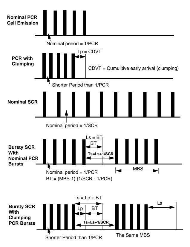
Figure 9.2 Illustration of Traffic Shaping Requirement in the FUNI IWF
