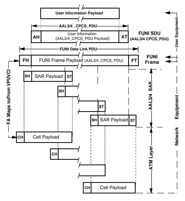
FH = FUNI Frame Header AH = AAL3/4 CPCS Header SH = SAR Header CH = Cell Header FT = FUNI/HDLC Frame Trailer AT = AAL3/4 CPCS Trailer ST = SAR Trailer Note: HDLC Flags are not shown
