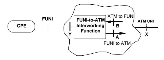
Figure 9.1 Reference Configuration for Traffic Management Specifications of the FUNI
