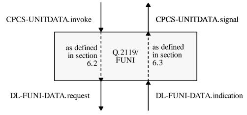
Figure 6.2: Relationship of AAL5-CPCS Signals and FUNI Service Primitives
