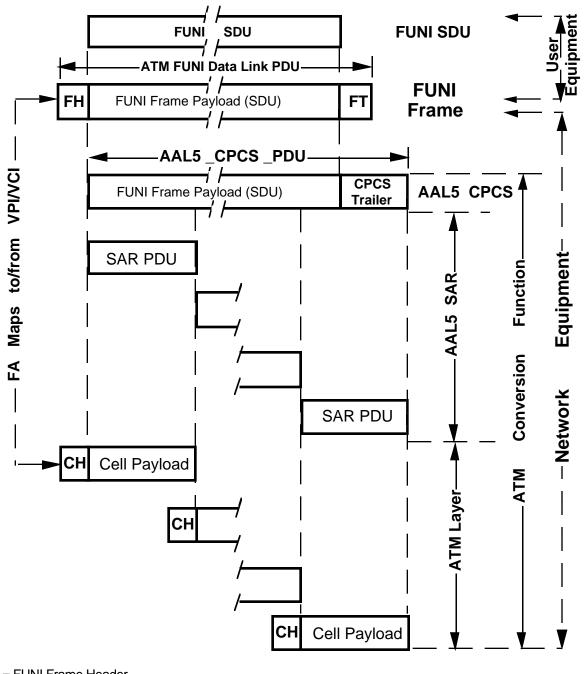
FH = FUNI Frame Header FT = FUNI/HDLC Frame Trailer = FCS CPCS = Common Part Convergence Sublayer CH = Cell Header Note: HDLC Flags are not shown
