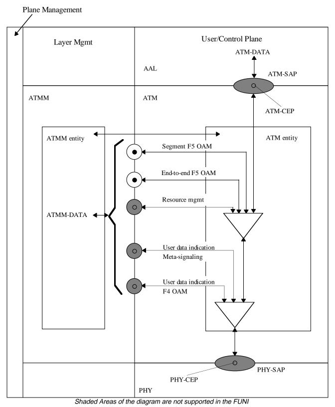
Figure 10.1: Interactions Between ATM- and ATMM-entities (Fig 4/I.361)
