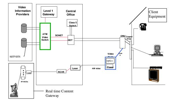
Figure B-2 Digital Baseband Network VoD Example
