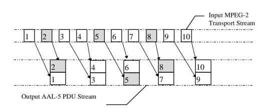
The specification does not require alignment of MPEG2-PCRs with AAL-5 SDUs - i.e. it is "PCR unaware".
