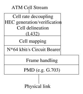
Observe that the mechanism for how to map ATM on a circuit bearer is not different from the general mechanism described in earlier specifications, e.g. in af-phy-0064.000 [2], "E1 Physical Interface Specification" and in G.804, [3] "ATM Cell Mapping into Plesiochronous Digital Hierarchy".
