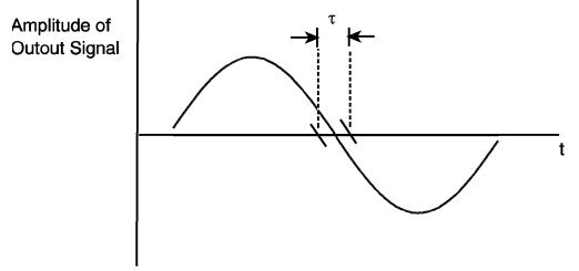
FIGURE 2-1 ILLUSTRATION OF TRANSMITTER JITTER
