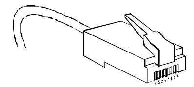
FIGURE 2-9 EXAMPLE OF A UTP-MIC MODULAR PLUG
