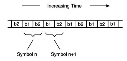
FIGURE 2-5 BIT-TO-SYMBOL MAPPING FOR 4-CAP
