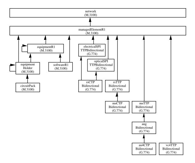
Figure 2-1a: Containment Tree Diagram (1 of 4)
