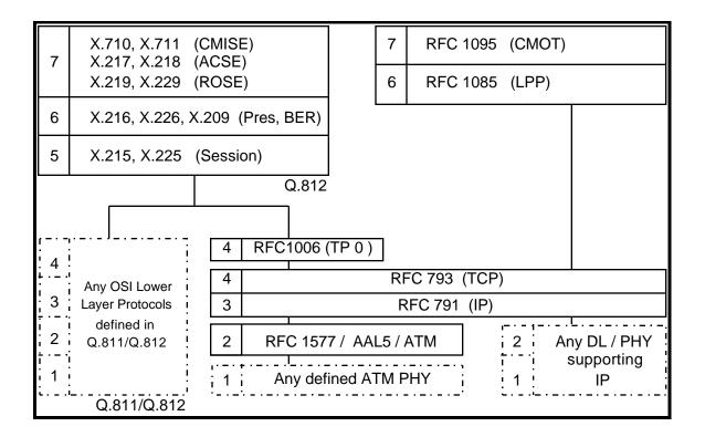
Figure A-1: Communications Stacks for the CMIP M4 Interface
