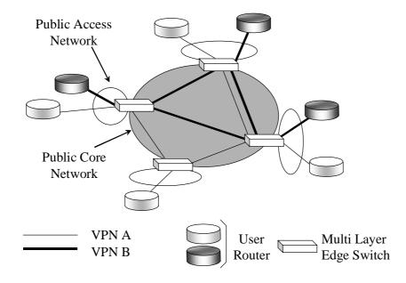
Figure 1: An Example of a Multi Layer VPN
