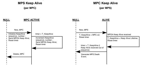
Figure 32 Egress MPC and MPS Keep-Alive State Machines
