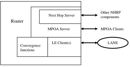
Figure 9 Router MPS Example
