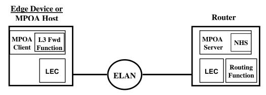
Figure 1 The Components in an MPOA System.
