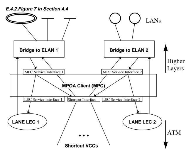
Figure 23 MPOA Edge Device MPC Example
