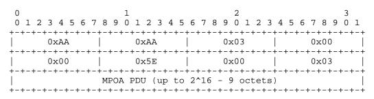
Figure 13 MPOA Control Frame Encapsulation
