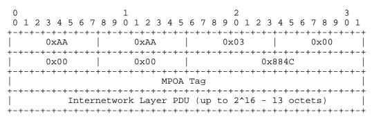
Figure 12 MPOA Tagged Encapsulation for Routed Protocols
