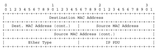
Figure 14 Ethernet IP Encapsulation
