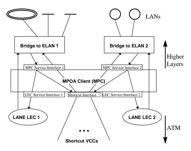
Figure 7 MPOA Edge Device MPC Example
