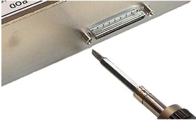
2. Remove the front panel (four screws).
