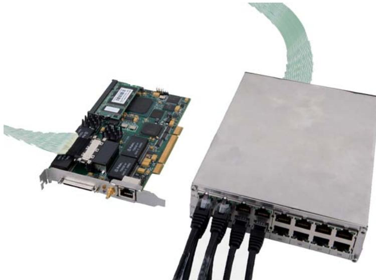
If the Pod is mounted external to the computer chassis you need to use the connector located on the card PCI bracket as shown in the picture below.
