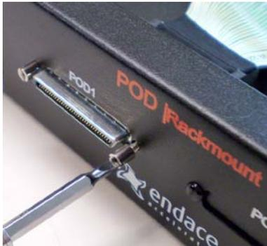
9. Mount the Pod PCB in the Pod chassis using four screws (supplied).
