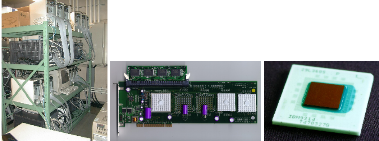
Figure 8: (a) MDGRAPE-2 and a host computer (left). (b) An MDGRAPE-2 board with two MDGRAPE-2 chips (middle). (c) An MDGRAPE-2 chip (right).
