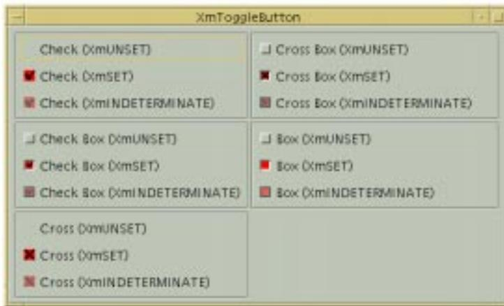
Figure 12-4: ToggleButton states and indicator appearance
