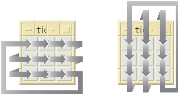
Figure 8-22: Keyboard traversal for the tictactoe program
