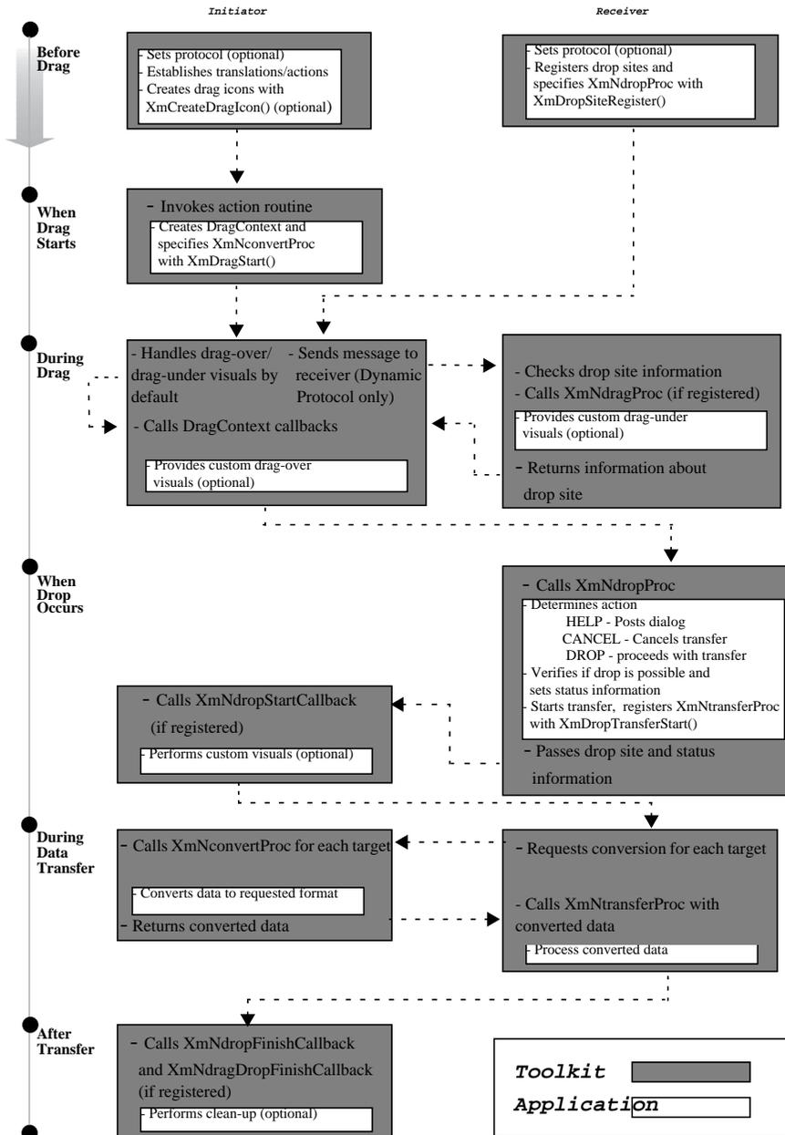
Figure 22-5: Drag and drop programming model
