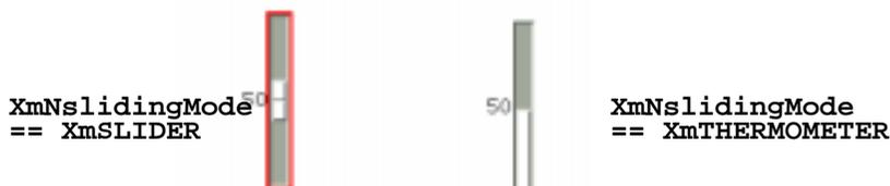
Figure 16-3: The XmNslidingMode resource and its effects
