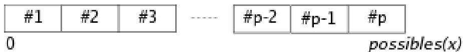
Figure 1: Each processor p gets an equal chunk ( possibles(x)/p ) of the keyspace from 0 to possibles(x) , where possibles(x) is the number of possible permutations for x .
