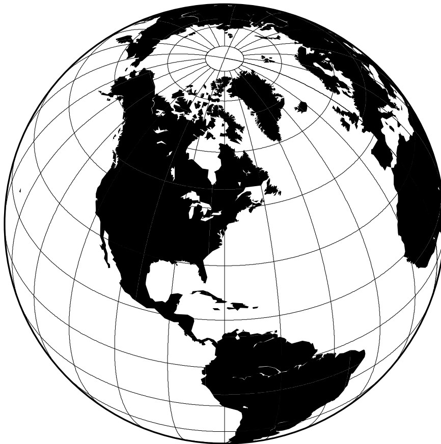
Figure 6.10: Hemisphere map using the Orthographic projection.
