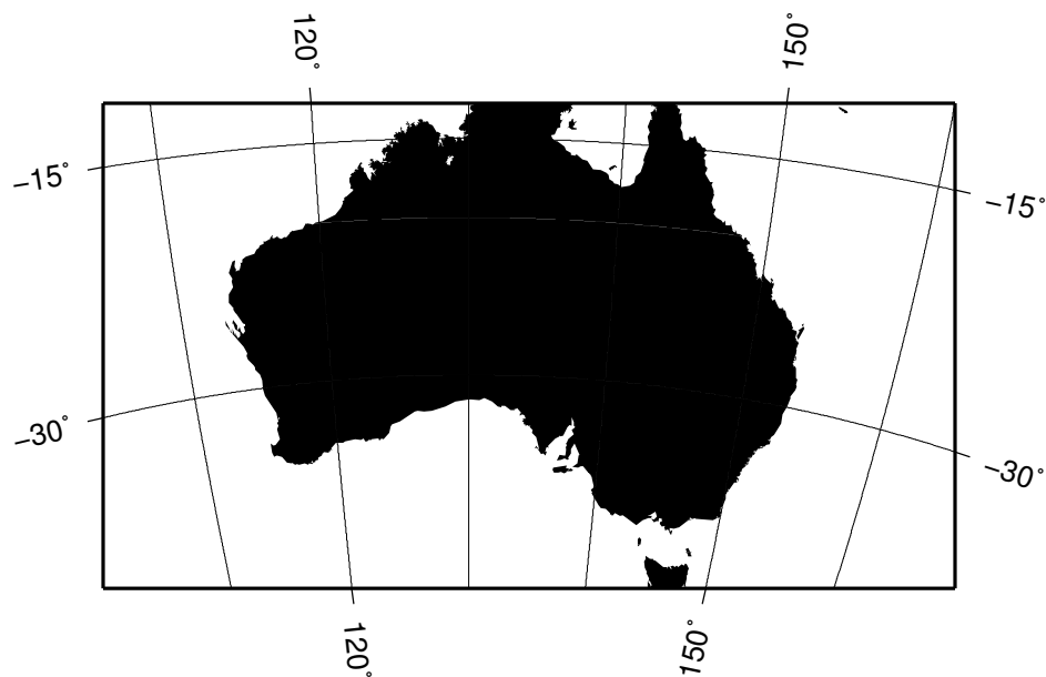
Figure 6.9: General stereographic conformal projection with rectangular borders.
